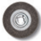
STEEL WIRE BRUSH Ø 250 mm x 60 mm, with very high wire drawing strength for highly efficient use, mounting hole Ø 51 mm. 0.2 mm thick wire for thin-walled pipes and profiles. 0.35 mm-thick wire for universal use. 0.5 mm thick wire for thick-walled pipes and profiles and great deburring results. Steel version
