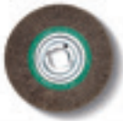
STEEL WIRE BRUSH Ø 250 mm x 60 mm, with very high wire drawing strength for highly efficient use, mounting hole Ø 51 mm. 0.2 mm thick wire for thin-walled pipes and profiles. 0.35 mm-thick wire for universal use. 0.5 mm thick wire for thick-walled pipes and profiles and great deburring results. Stainless steel version
